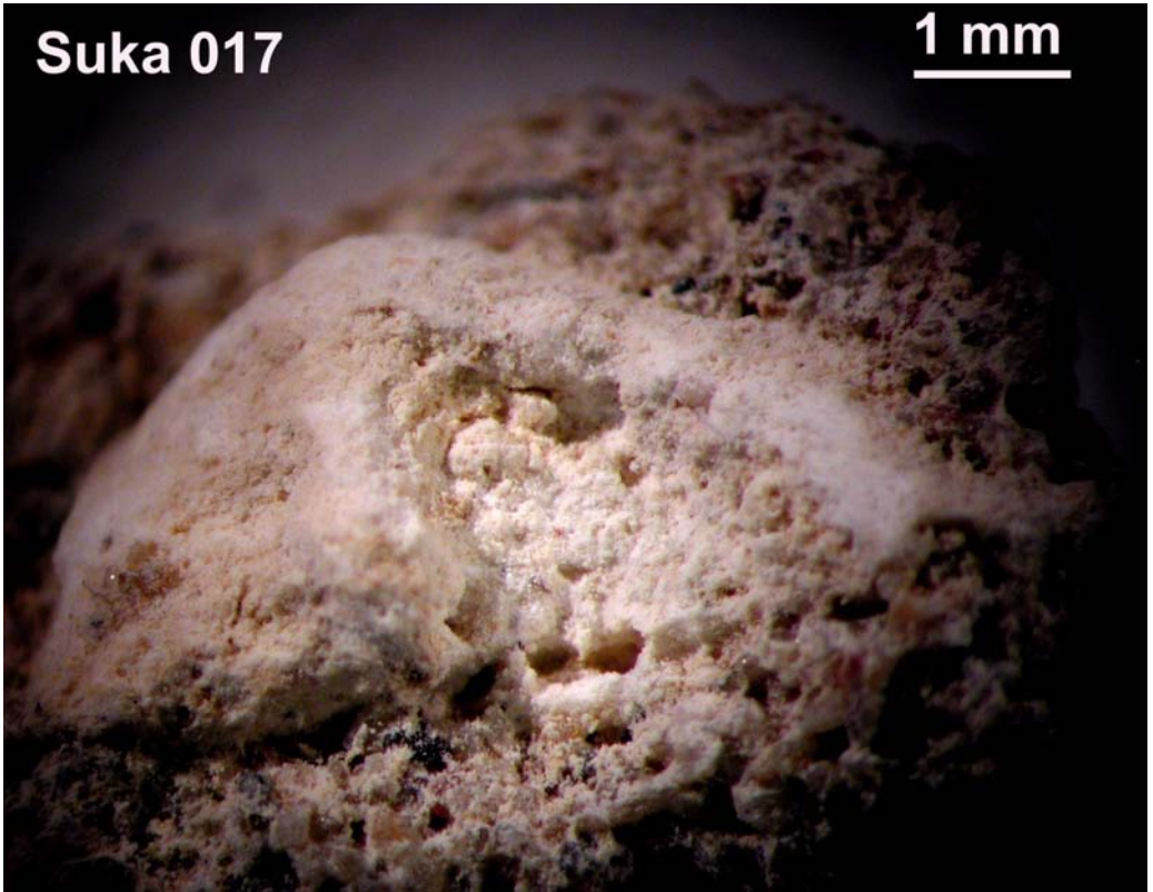
Figure 10 A piece of mortar from the church of Sund (sample Suka 017). Percolating waters have dissolved some of the binder, and new calcites have formed a crust around a lime lump. In voids inside the lump, still younger, light efflorescent calcites have grown.
